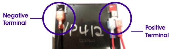
**TIP:** You may need to use a pair of pliers with electrically insulated handles. You may need to wiggle the connector slightly for it to come loose. The red wire connector (positive terminal) may have two connections. This connector will slide off the terminal the same way as the black wire connector (negative).
