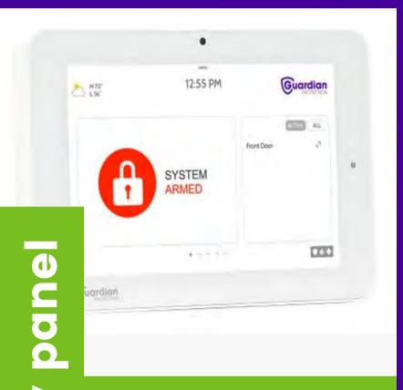
The brain of your security system that controls everything. This is where you enter your code to arm and disarm the system. Most modern panels are touchscreens, and some include features like cameras and glassbreak detection. Sometimes referred to as a hub, keypad, or control panel.
